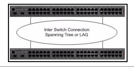
In the alternate integrated device configuration, bridge priority is less significant but other factors may add to complexity. In particular, link sizing becomes an issue if there are not enough Gigabit Ethernet aggregation ports. If a link aggregation group (LAG) is used, flow distributions must be understood to ensure correct behavior.
